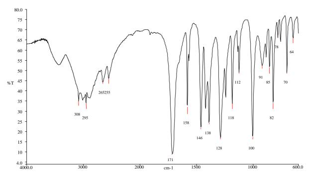
Fig. 11 Infrared spectrum of dicamba
